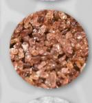
**Level 4:** High Density Garnet Media High hardness, high density filter media, effectively filters and provides a high quality support bed for this system.
